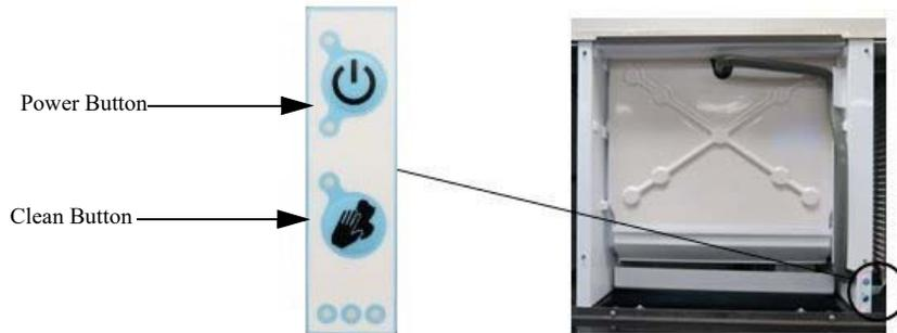
4. Once the ice machine has completed its harvest cycle, the POWER light will go to solid red (OFF mode).
