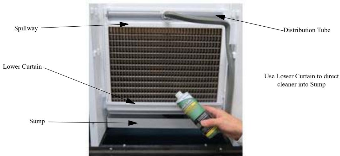
10. The machine will remain in the WASH cycle for 15 minutes.
